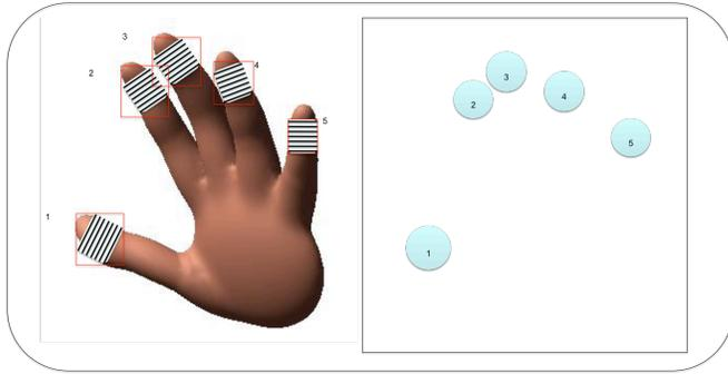
Figure 2. Picture showing the finger wraps and our original design. Initially we planned to use barcode like strips on the wrap to allow identification of individual finger, but we did not have the time to implement that yet.
