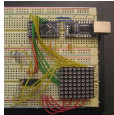
Figure 1. Picture of our prototype of the Multi-touch LED Matrix Display
